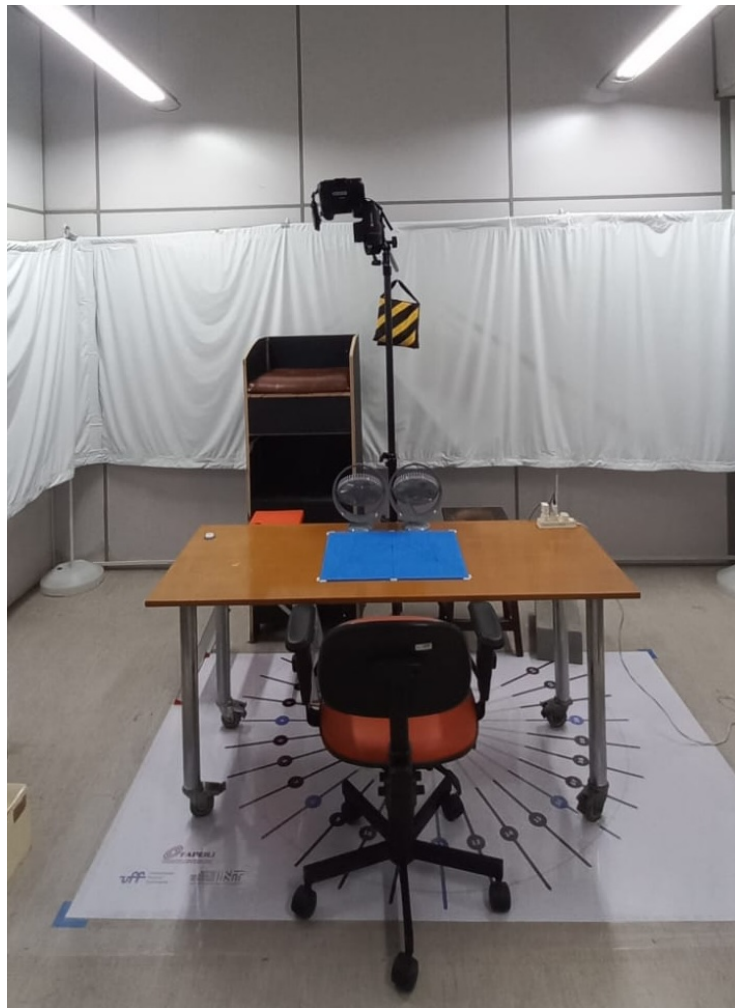
Figure 2. Acquisition environment: thermal camera mounted on tripod, EVA plate (blue) on the table, USB fans positioned in front of the plate, and a white background curtain to homogenize the optical environment. The volunteer is seated facing the table during the exam.
