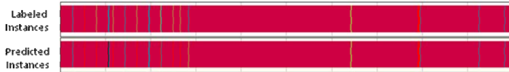
Figure 8 - VISUALIZATION OF THE LABELED INSTANCES IN TIME AND THE NEURAL NETWORK PREDICTION. RED REPRESENTS INSTANCES LABELED AND/OR PREDICTED AS NORMAL AND OTHER COLORS REPRESENT INSTANCES LABELED AND/OR PREDICTED AS OTHER EVENTS (PUMP START, VALVE ADJUSTMENT AND/OR BATCH CHANGES).
