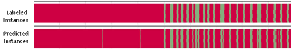
Figure 7 - VISUALIZATION OF THE LABELED INSTANCES IN TIME AND THE NEURAL NETWORK PREDICTION. RED REPRESENTS INSTANCES LABELED AND/OR PREDICTED AS NORMAL AND GREEN REPRESENTS INSTANCES LABELED AND/OR PREDICTED AS A LEAK.
