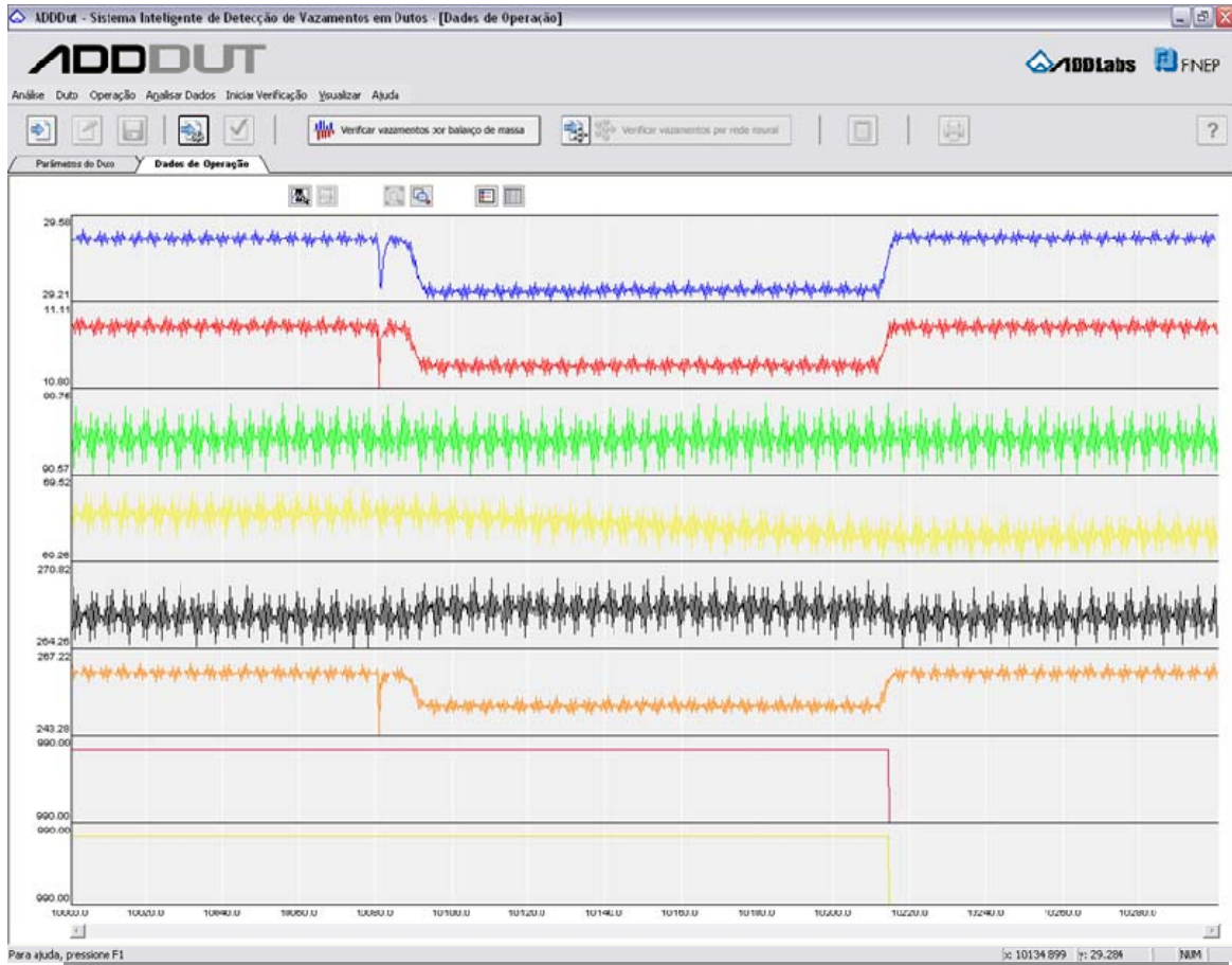
Figure 3 - VISUALIZATION OF THE SIGNALS IN TIME. FROM TOP TO BOTTOM: FLOW RATE (INPUT AND OUTPUT), TEMPERATURE (INPUT AND OUTPUT), PRESSURE (INPUT AND OUTPUT) AND DENSITY (INPUT OUTPUT).
