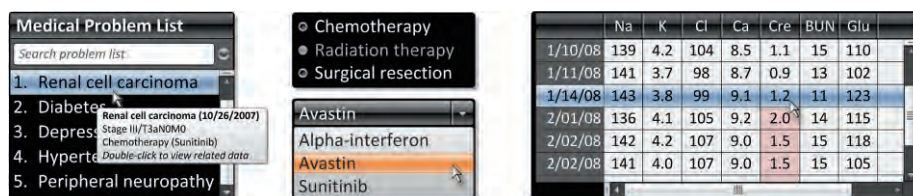
Figure 4.1: Lists and tables are a common graphical component used to present clinical data. From left to right: a patient’s medical problem list is shown using a searchable and scrollable list, with tooltips presenting more specific information; radio buttons, checkboxes, and combo boxes are used to provide selection capability from a fixed set of options; and table are often used to present multivariate data for comparison, such as with lab panels.
