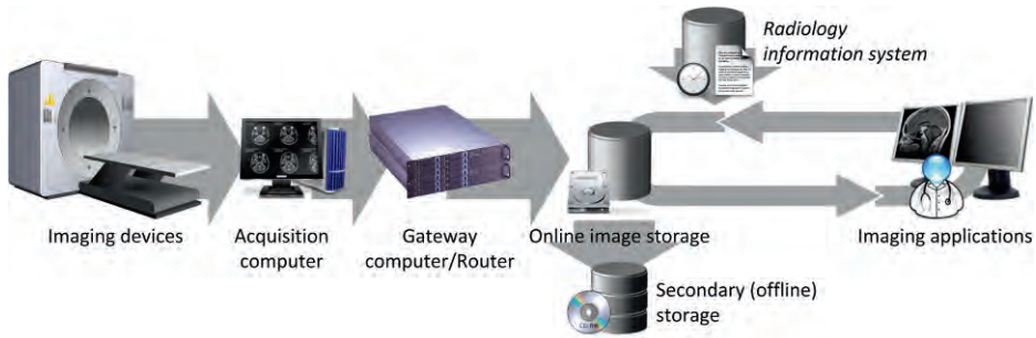
Figure 3.2: Components of a picture archive and communication system (PACS). Arrows between the different parts illustrate data flow.
