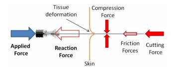
The model proposed for the needle insertion **before** a tissue puncture is:
