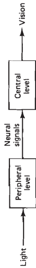
Figure 7.14 Human visual system as a cascade of two systems. The first system represents the peripheral level of the visual system and converts light to neural signals. The second system represents the central level and processes neural signals to extract necessary information.
