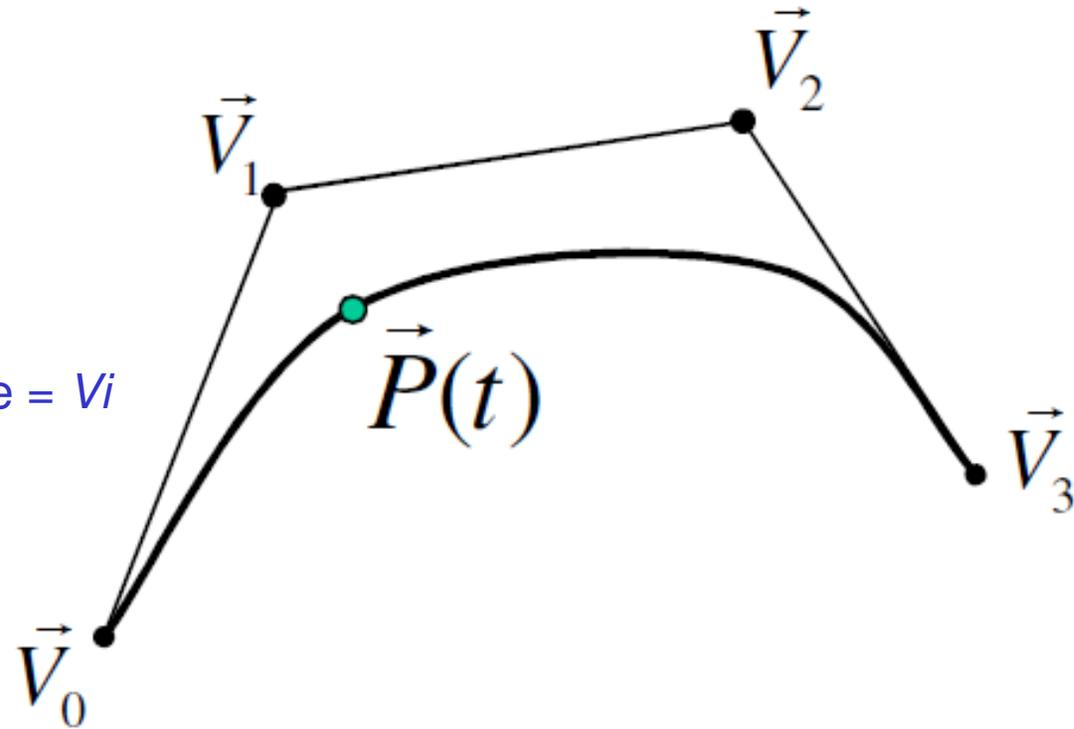
$$\vec{P}(t) = (1-t)^3 \vec{V}_0 + 3(1-t)^2 t \vec{V}_1 + 3(1-t)t^2 \vec{V}_2 + t^3 \vec{V}_3$$
