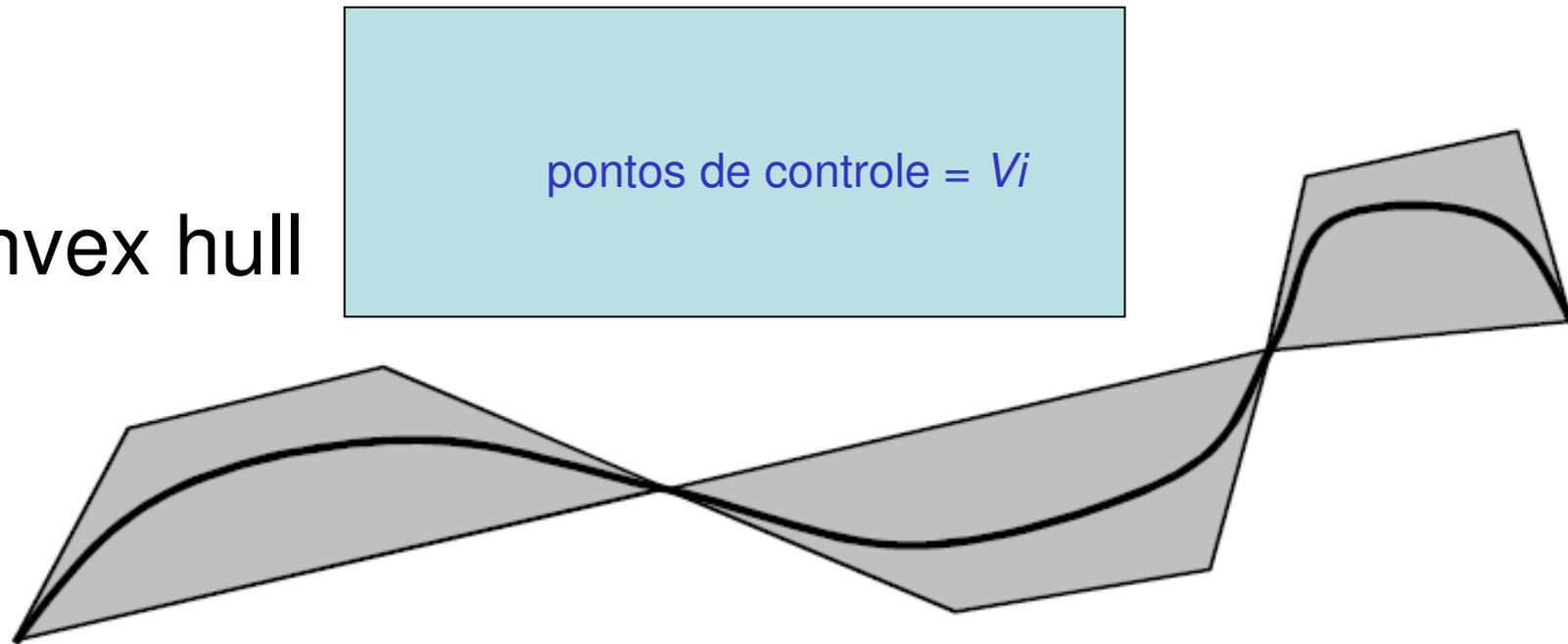
$$\vec{P}(t) = \sum_{i=0}^n \alpha_i \vec{V}_i \quad \text{com} \quad \sum_{i=0}^n \alpha_i = 1$$
